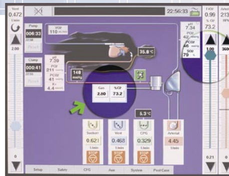
Central control for the electronic gas blender/O 2 analyzer
