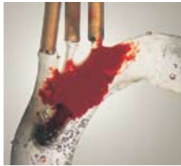
Jetting action typical of standard aortic cannulae.
